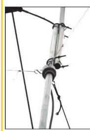
One problem that I discovered with the 6m beam, was that it was in a bad location with respect to the house. It was not above the roof, so the house cast a bit of a shadow and raised the noise floor. I was able to get K2LIM on 2m and 1.25m, but I could just barely hear them on 6m. Something to improve for next time.
